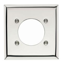
Two Gang Power Outlet Receptacle Opening, 2.1563 hole for 2.125 diameter device - 4 mtg. holes, Smooth Metal.
