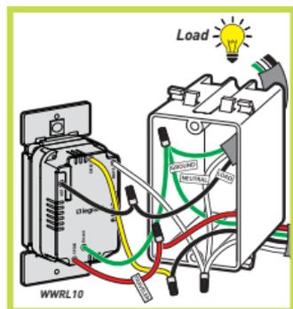
**NOTE:** To wire Smart Switch to the load side of the circuit. Connect the HOT wire on the switch to load that is being controlled.
