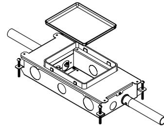
**WARNING:** Pour concrete to 1/16" (1.6 mm) above box housing. Pours of 1/4" (6.4 mm) or more over box housing will make it difficult to break out the mud cap and cause excessive concrete spalling.
