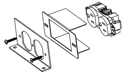
**NOTE:** Use insulator provided with the following catalog numbers, installed as shown: RFB2DP, RFB2GFI.
