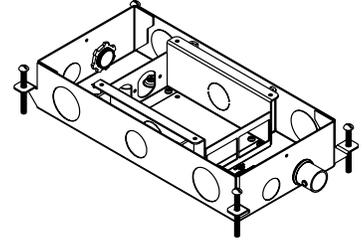
**NOTE:** Box is supplied with tunnel bracket, tunnel blocks and device mounting brackets installed. If the same service is to be used in both compartments, it will be necessary to remove one or both of the tunnel blocks to allow for pass-through of the service wiring. The tunnel blocks are accessible by removing the tunnel support. The installer may do this either pre- or post-pour.
