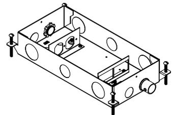
**NOTE:** Box is supplied with tunnel bracket, tunnel blocks and device mounting brackets installed. If the same service is to be used in both compartments, it will be necessary to remove one or both of the tunnel blocks to allow for pass through of the service wiring. The tunnel blocks are accessible by removing the tunnel support. The installer may do this either pre- or post-installation.
