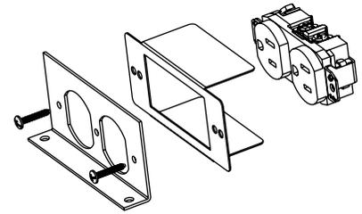
**NOTE:** Use insulator provided with the following catalog numbers, installed as shown: RFB2DP, RFB2GFI.
