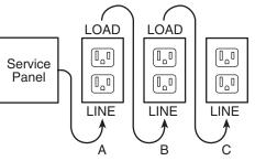
Placing the GFCI in position A will also provide protection to "load side" receptacles B and C. On the other hand, placing the GFCI in position C will not provide protection to receptacles A or B. Remember that receptacles A, B, and C can be in different rooms.
