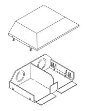
The Entrance End Fitting is used to provide an end feed to Access<sup>™</sup> 5000 Raceway with 1/2" or 3/4" conduit. Installation should be as shown with side walls of the Fitting Base and Raceway Base aligned.
