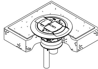
**CAUTION:** Poke-Thru cannot be rotated in hole after inserted into floor.
