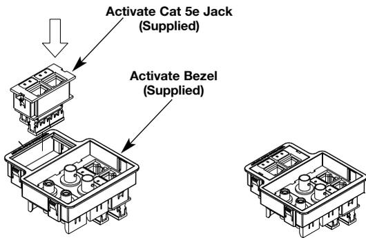
**Pass & Seymour ACTIVATE Bezel and Communication Jack (Supplied with AMD8ATC & AMD8CTC Units).**
