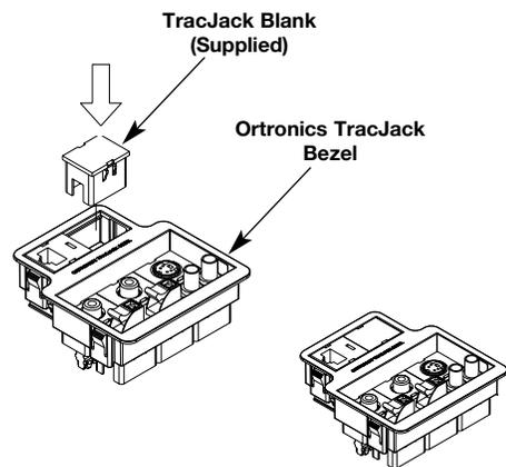
**CAUTION:** Empty communication ports must be closed off with foam blocks, or TracJack blanks to maintain Fire Classification.
