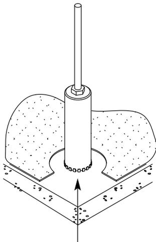
4" [102mm] Diameter Core Drill
