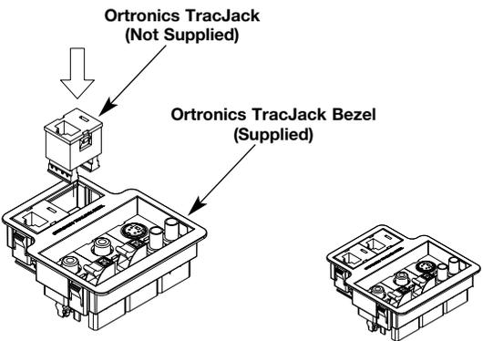
**Ortronics TracJack Bezel & Communication Jack (Bezel Supplied with AMD8ARTTC and AMD8CRTTC TracJacks Sold Separately).**
