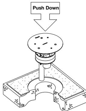
**CAUTION: Poke-Thru cannot be rotated in hole after insertion into floor.**
