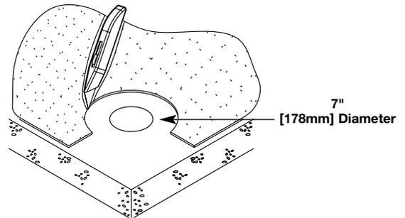
**CAUTION: For tile installations up to a maximum of 3/4" [19.1mm] thick.**
