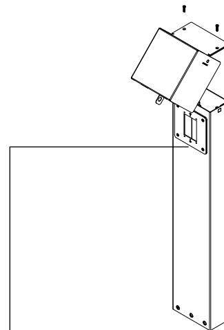
For locking feature the faceplate will need to be replaced with a locking tab version
