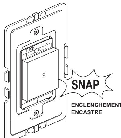
**NOTE** - If you need to remove switch after snapping into frame, first remove frame from wall box to access the four locking tabs on the back of the switch. Insert a flat screwdriver to depress tabs as you apply pressure to push switch out.
