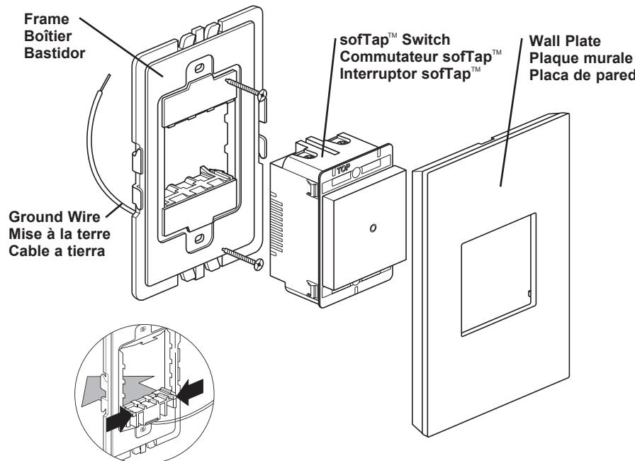
**Remove spacers from the frame.** Since this switch fills the frame completely, you will not need the spacers. From the back of the frame, pinch the tabs on the spacer to release.
