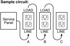
Placing the GFCI in position A will also provide protection to "load side" outlets B and C. On the other hand. placing the GFCI in position C will not provide protection to outlets A or B. Remember that outlets A. B. and C can be in different rooms.
