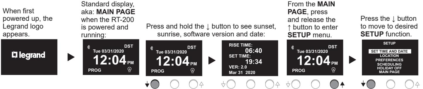
**NOTE:** Once in **SETUP** menu, the ↓ button moves to the previous menu or decreases the value, the ↑ button moves to next menu or increases the value. The **center** button confirms the selected variable.
