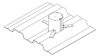
NOTE: Insure that all gaps between deck and tube are sealed completely.
