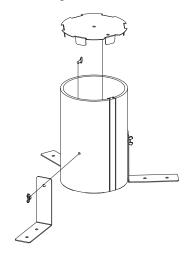
STEP 2. Attach Pre-Pour Sleeve assembly to the Deck.
