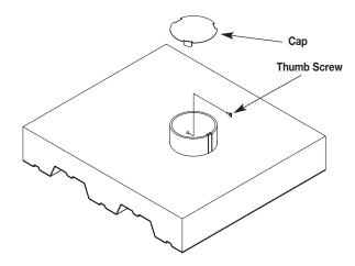
**STEP 5.** Tap Binding Key out of Tube. Once the Binding Key is removed, the Tube will collapse inward and can be removed from the Hole.
