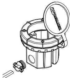
5. Orient the box to the desired rotation and push into the hole. The box will not turn once installed so make sure the receptacle will be parallel or perpendicular with any adjacent walls.
