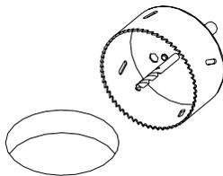
2. For a flush installation in hardwood or tile floors with the 895T or 896T series covers - cut a 4 5/16" [109mm] diameter, 1/8" [3.2mm] deep step in the final floor covering.
