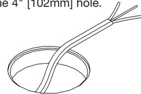
**NOTE:** For air handling spaces allowed for that application. See NEC 300-22(C). For communications applications, type CMP communication plenum cable is required in raised floor plenums when wiring methods as described in NEC article 300-22(C) are not followed.
