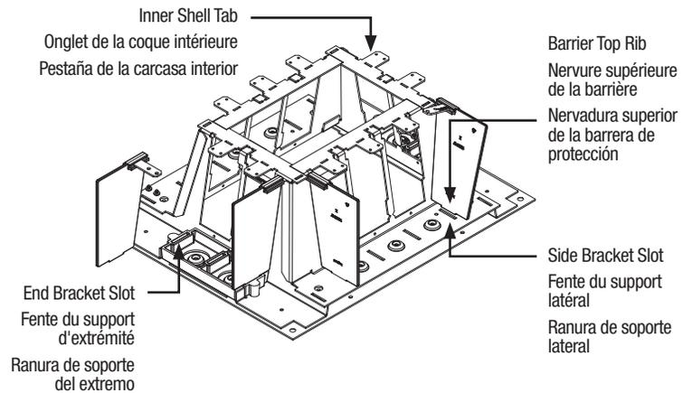
**3** Roll the barrier and mounting clip in place and secure to the innershell tab with the (2) mounting screws provided.
