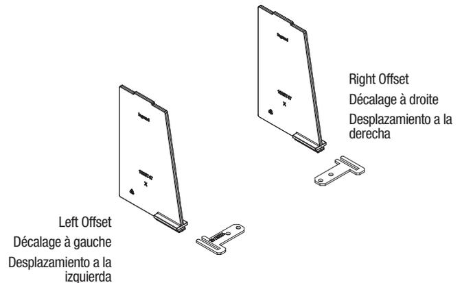
**2** Insert the rib on the top edge of the barrier into the slot located at the top of the slide or end bracket.
