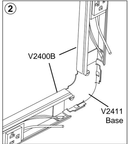
Insert V2400B Base under each tongue of V2411 Base. Mount V2400 Base and Cover per system instruction sheet.
