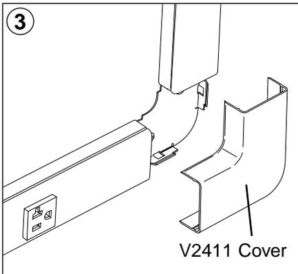
Snap V2411 cover over raceway at corner.
