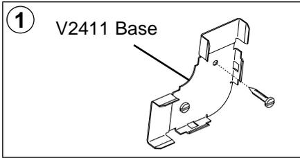
Mount V2411Base to wall using two No. 10 Pan Head screws.
