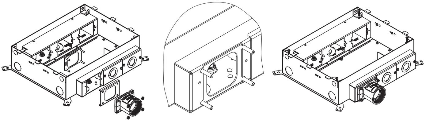
**Step 6.** Complete the installation by attaching 2 inch conduit to the Hub.
