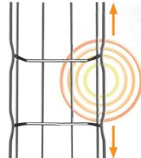
The steel structure of Cablofil tray reduces Electromagnetic Interference (EMI) and stray static charges.
