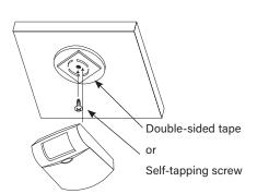
Sensor mounts under desk or binder bin with double-sided tape or self-tapping screw
