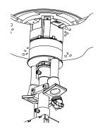
Step 4. Attach conduit to fitting and pull wire or cable through raceway.
