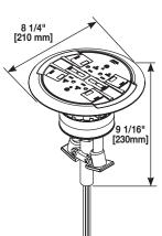
Assembled Unit – Unit includes four prewired 20A receptacles. Each duplex can be wired as a separate circuit. The duplex can be wired as a standard receptacle or isolated ground. Wiremold Open System unloaded inserts to accept four discrete keystone \* connectors from most manufacturers are provided.
