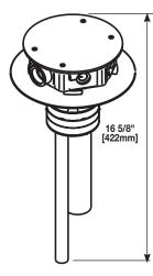
Assembled Furniture Feed Unit – Complete with hexagonal service head. Service head has one 3/4" threaded conduit hub and five rubber grommets. The service head includes scrub water gasket. Unit is supplied with one 1 1/4" trade size conduit stem and one 1/2" trade size conduit stem to feed power and communication services.
