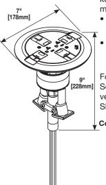
Assembled Unit – Prewired 20A duplex receptacle can be wired as standard duplex or isolated ground. Wiremold Open System unloaded inserts to accept two discrete keystone connectors from most manufacturers are provided.
