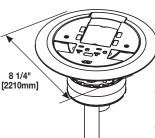
**Assembled Unit** – A/V device includes one prewired 20A duplex receptacle which can be wired as a standard receptacle or isolated around.
