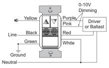
Note: Requires Class 1 wiring for 0-10V dimming.
