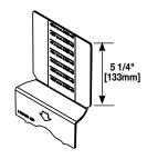
**PVC Floor Box Divider Plate -**Used to isolate power and communication compartments. Graduated cubic inch markings are marked clearly on the divider and correspond directly to the cubic inch markings on the interior of the box. Cuts easily with a utility knife. Supplied with a receptacle plate that completes separation of power and communication services. One divider required for dual- service activation.
