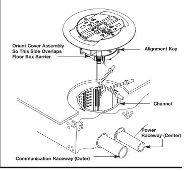
Step 12. Wire and install communication jacks as required using one of the following methods shown below.
