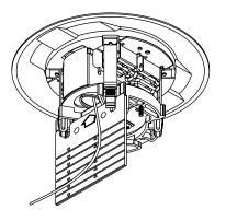
**Step 9.** Remove slide cover to access communication raceway.
