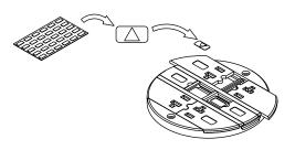
The orange triangle shall only be placed on devices that are wired for isolated ground (see NEC 250-146 (d)).
