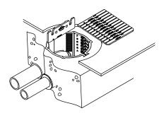
Actual distance between top of box (after cutting away excess) and top of divider is 2 3/8" [61mm]. If uncertain where to cut divider for regions between letters (through horizontal bar), cut divider to measure a minimum of 2 3/8" [61mm] below floor level. Can be slightly less if thick floor covering is used.
