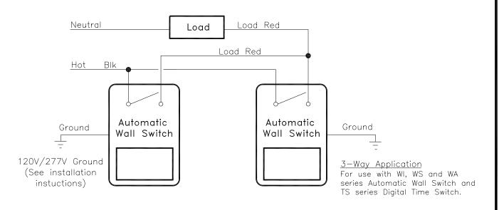
\*When these switches are wired in a three—way wiring configuration they will only operate as three—way switches if they are left in automatic mode. If one switch is turned off, the lights will not come automatically on until that switch is turn back to the automatic position. We recommend other control options for multi—way switching applications.
