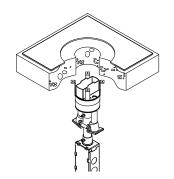
Remove poke-thru unit from hole.
