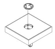
Step 4 Push in proper abandonment plug. For 3" core hole, use ABPLUG3 For 4" core hole, use ABPLUG4 For 6" core hole, use ABPLUG6 For 8" core hole, use ABPLUG8
