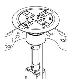
For ABPLUG3 & ABPLUG4: Remove slide holder assembly and the internal gasket. Disconnect power and communications devices and remove flange.
