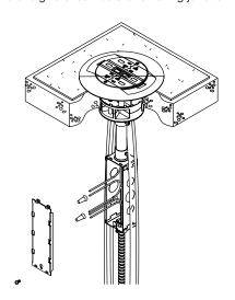
Step 2. Remove two screws and slide holder.
