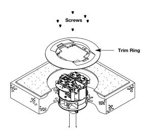
**Step 4.** Pull receptacles and receptacle brackets out of Poke-Thru device.
