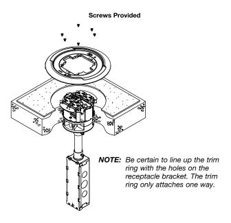
**Step 7.** Place gasket support on receptacle bracket. Place internal gasket on gasket support and press around edge to seat the gasket into the groove in the trim ring.
