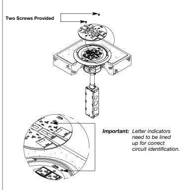
**Step 9.** Make electrical connections in junction box according to wiring diagram.
