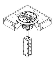
**NOTE:** Factory supplied junction box shown. Junction boxes must be located in an accessible location. Poke-Thru devices with an "LJB" or "LJB25" suffix are supplied without a junction box (supplied by others).
