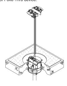
**Step 5.** Guide replacement receptacle brackets into place. Direct wire leads through indicated opening to junction box below.
