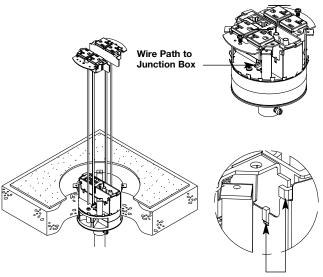
Important: Receptacle bracket slides into the tabs shown here.
