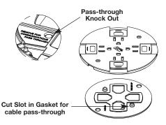
**4.** Pull communication cables through box. Route one of the cables around the receptacle for cable egress opposite the communication compartment in the floor box. Reattach slide cover with (2) #6 screws. Pass through cabling must pass through internal gasket and slide cover.
