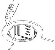
4. Attach conduit to conduit fitting, pull wires and push activation into floor box until firmly seated on floor.
