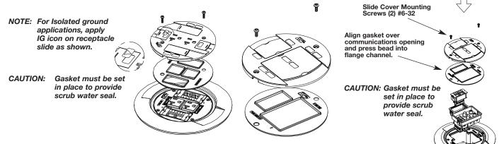
CAUTION: Receptacle supplied with this activation is not suitable for direct field wiring. Contact manufacturer for replacement. Field modifications will void UL Listing. Replacement receptacle is limited to this manufacturer's catalog No. RC37REC.
