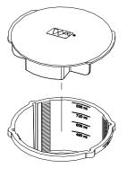
For dual service applications, slide partition onto the slots located on the inside of the box and mark the partition 2" [51mm] below the top of the box. Volume of power compartment is reduced by the first legible calibration.
