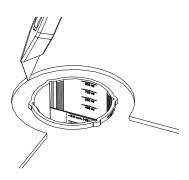
4. Remove the slide cover, gasket, and trim flange to access the communications compartments.
