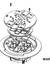
WARNING: Receptacle mounting means not grounded. Grounding wire connection required. For isolated ground wiring, connect ground leads to a separate isolated grounding conductor (see NEC 250-146(d)).
