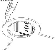
**2.** Remove the slide cover and gasket to access the communications compartments.
