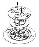
7. Align gasket over receptacle and press bead into flange channel.
