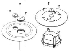
**3.** Attach the necessary conduit fittings to the flange. Connect the flexible conduit and wires. All splices must be made in the box below the cover adapter.
