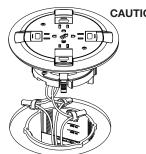
CAUTION: Receptacle mounting means not grounded. Grounding wire connection required. For isolated ground wiring, connect ground leads to a separate isolated grounding conductor (see NEC 250-146(d)).
