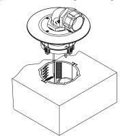
CAUTION: Flange must be grounded. Connect attached grounding conductor to system ground. Maximum circuit conductor size shall not exceed No. 12 AWG.
