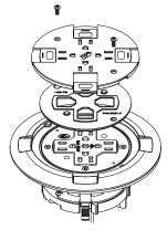
**3.** For communication cable pass-through, remove the egress knockout(s) located on the underside of the cover.
