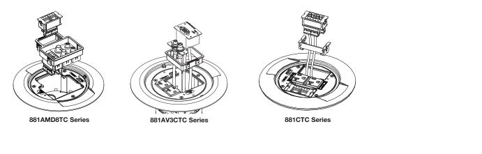
7. Align gasket over receptacle and press bead into flange channel. Reattach slide cover with two #6 screws.
