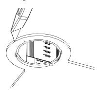
2. Remove the slide cover and gasket to facilitate the routing of the communication cables.
