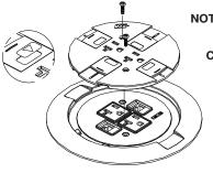
NOTE: For Isolated ground applications, apply IG icon on receptacle slide as shown.
