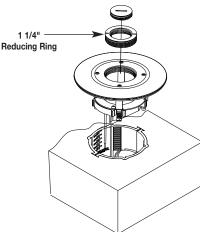
**3.** Attach a 2" or 1 1/4" trade size conduit fitting (not supplied) to the flange. If a 1 1/4" trade size fitting is used, insert the 1 1/4" reducing ring supplied before inserting the fitting.
