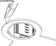
4. Push the activation into the floor box until firmly seated against the floor.
