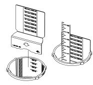
**3.** Remove the partition and break off the top portion at the first calibration below the mark made from step 2. Reinstall the partition with the small compartment being the communications side.
