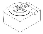
**2.** Remove necessary screw plugs from the flange.
