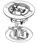
WARNING: Receptacle mounting means not grounded. Grounding wire connection required. For isolated ground wiring, connect ground leads to a separate isolated grounding conductor (see NEC 250-146(d)).
