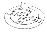
6. Wire and snap communication jacks into flange.
