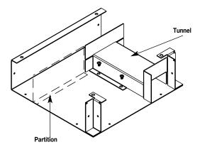
**NOTE:** Using tunnels reduces your overall wire fill capacity by 50% due to reduced area for wires in the system as a whole.
