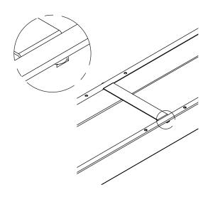
**Step 4** To attach cover, place palnut clip over holes on top side of duct as shown. Position cover and secure into place using #10-32 machine screws provided.
