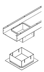
**Step 4** Adjust depth of drop out by loosening and tightening the four #10-32 taptite screws on the side of the unit until it sits flush as desired. Cut desired hole size into drop out coverplate. Place grommet supplied around field cut hole.
