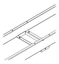
**Step 4** Attach the other duct body to drop out using screws and coupling angles provided. Run wires, wire retainers and close duct bodies as necessary.
