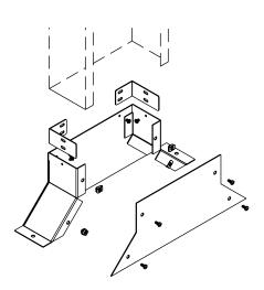
Step 1 For VA Risers – Attach riser to duct body using coupling angles provided with duct body and attach to trench body using screws provided through tabs provided with the VA body.
