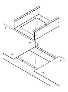
Step 2 For Flush to Surface Transition – With coverplate area prepared, apply grommet to all sharp edges, place wires and wire retainers, and attach transition with planut clips and #10-32 machine screws provided.
