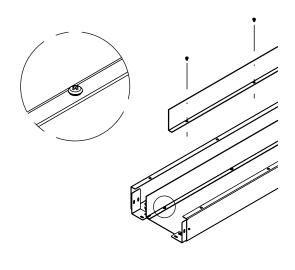
Step 3 Place wires into duct and then slide wire retainers into place (wires not shown for clarity). The wire retainer fits in slots located at the end of each duct body and in the middle of a 60" [1,524mm] body.
