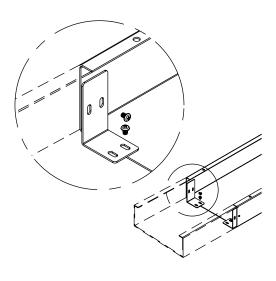
Step 2 With bodies connected and mounted to wall with screws, place partitions into duct as necessary making sure wire fill requirements are followed as per NEC (Wire fill information is also located onlast page of instruction sheet).
