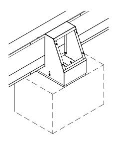
**Step 4** Place wires and attach cover onto body with screws provided.
