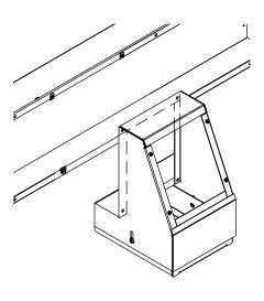
**Step 3** Attach cabinet connector to unit by adjusting bottom to sit flush with cabinet and then fasten with appropriate screws (provided by others).
