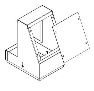
Step 2 Fasten unit to duct body. Holes for connection will need to be drilled in the straight body flanges as necessary using a 9/32" [7.14mm] diameter bit. Use the holes in the sweep cabinet connector as a guide to drill the holes. Place palnut clips over drilled holes. Re-position cabinet connector to line up with palnut clips. Secure into place using #10-32 machine screws provided.
