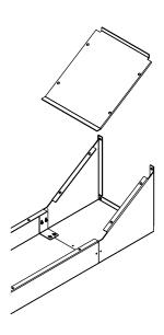
Step 2 For Sweep Tees – Attach unit to the other duct body using #10-32 machine screw and palnut clips provided. Refer to instructions shown in step 2 of previous page for attachment method.
