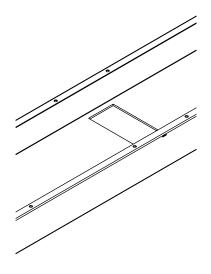
Step 2 Drill four holes with a diameter of 9/32"
