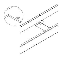
Step 3 Place drop out unit into body and screw into place with palnut clips and #10-32 machine screws. Installation is similar to that of a coverplate.
