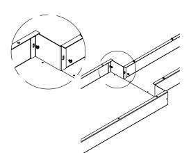
**Step 1 For End Closures** – Fasten closure to body of duct using screws provided. The closure should be attached just like a coupling angle.
