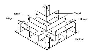
**NOTE:** Using tunnels reduces your overall wire fill capacity by 50% due to reduced area for wires in the system as a whole.
