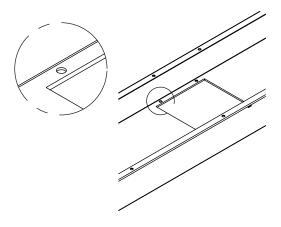
**NOTE:** File all sharp edges and burrs on the wallduct that may cut wire insulation.
