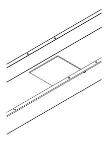
Step 2 Drill four holes with a diameter of 9/32" [7.144mm] to match with ceiling drop out mounting holes. This can be best achieved by placing the drop out onto duct body and marking with a marker or pencil. These are the locations for the palnut clips and machine screws.
