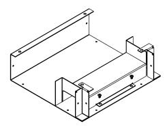
Step 2 For 2 Compartment T-Unit Tunnels – If the partition of the adjoining Wallduct sections have not been installed prior to the assembly of the T-unit tunnels/bridges, cut the partition long enough to extend into the T-Unit and abut the tunnel/bridges as shown.
