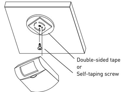
Sensor mounts under desk or binder bin with double-sided tape or self-taping screw
