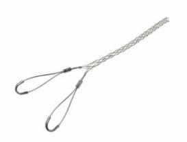
Standard-duty, Closed mesh, Double eye grips. Cable diameter -0.500-0.610-inch, Bale length - 4-inch, Mesh length - 11-inch, Break strength - 770 lbs.
