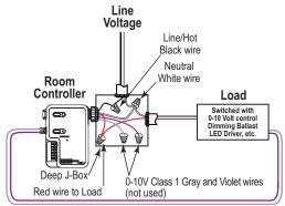
0-10V Class 2 Dimming control wires
