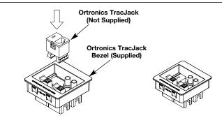
Ortronics TracJack Bezel & Communication Jack (Bezel Supplied with AV3ARTTC and AV3CRTTC, TracJacks sold separately).
