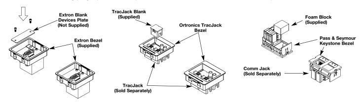
CAUTION: Empty communication ports must be closed off with foam blocks, TracJack blanks or Extron Single and/or Double MAAP blanks to maintain Fire Classification.
