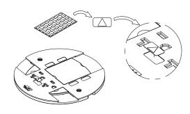
NOTE: The orange triangle shall only be placed on devices that are wired for isolated ground. See NEC 250-146(d).
