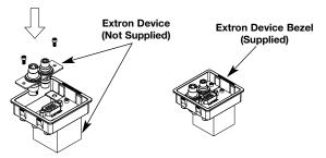
NOTE: This Bezel Accommodates (1) Single and (1) Double or (3) Single MAAPs (Mini Architectural Adapter Plates) Extron Devices.
