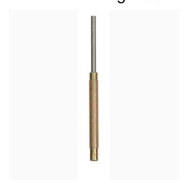
This long-style Pin Punch from Klein Tools is great for driving out and removing pins and keys. It features a soft head that will mushroom instead of chip for added safety. The knurled handle provides better grip.
