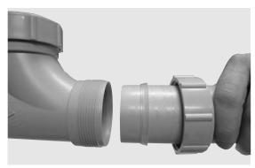
\*If you are working on a job that has the old translucent nonelastic olives, consult your "heat olive" Technical Bulletin or call IPEX Customer Services for technical information. 6. Apply IPEX Acid Waste Lubricant or IPEX approved petroleum jelly to both the thread and the elastolive then push the pipe squarely into the fitting.
