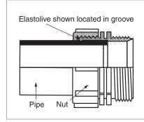
Once engaged in the groove, the elastolive virtually becomes part of the pipe and when the nut is tightened, the pipe is locked into the fitting.
