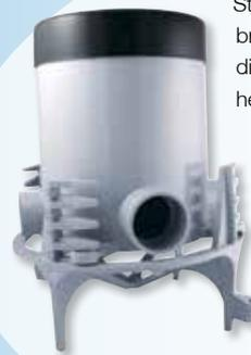
This simple yet innovative Round Floor Box Stand is equipped with several height brackets which accommodate the different rebar and post-tension cable heights and slab depths found from jobsite to job-site. When installed together, the Floor Box and Stand can be used in 5-1/2" to 10" slab depths.
