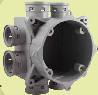
Approved for support of ceiling fans up to 35 lbs. and luminaries up to 50 lbs, slab boxes are supplied as a fully assembled one-piece unit. All molded connectors have 360° locking tabs that exceed UL and CSA requirements for pull-out.
