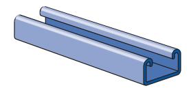
Wt/100 Ft: 25 Lbs (38 kg/100m) Allowable Moment 170 In-Lbs (20 N•m) 19 Gauge Nominal Thickness .040" (1.0 mm)
