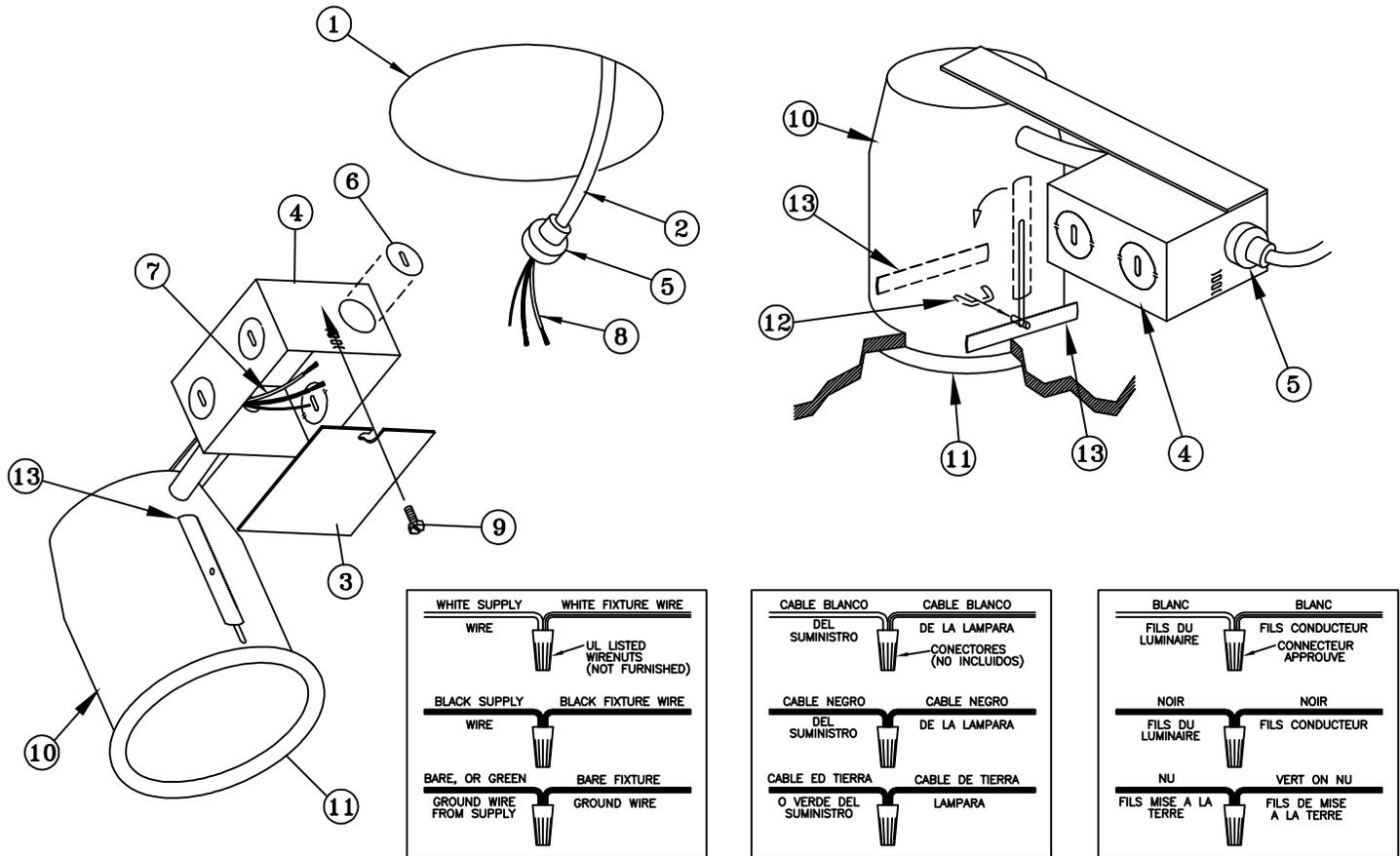
1.- Cut a 4 1/2 inch diameter Hole (1) in Ceiling and pull electrical Supply Cable (2) down through opening.
