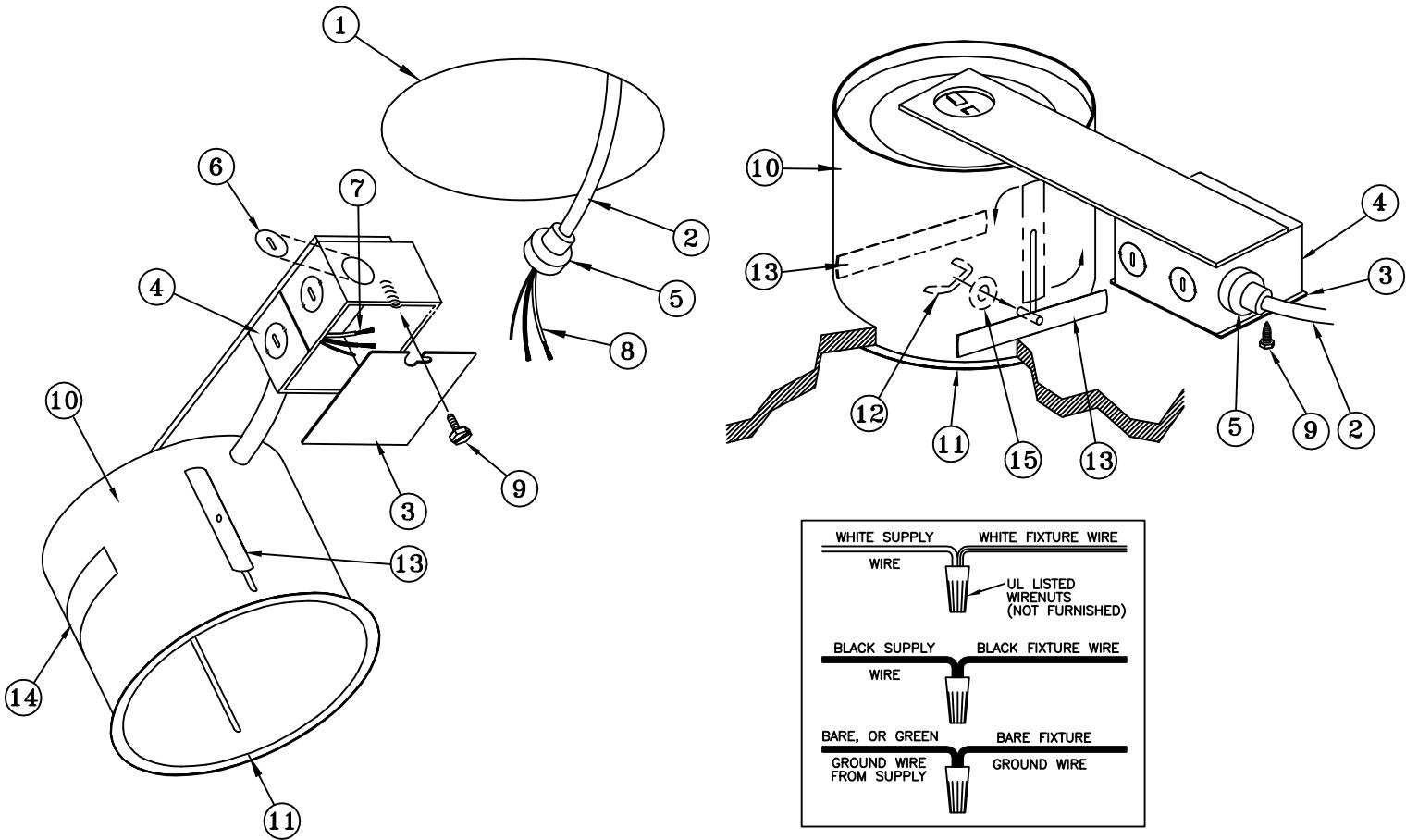
1.- Cut a 6 5/8 inch Diameter Hole (1) in Ceiling and pull Electrical Supply Cable (2) down through opening.
