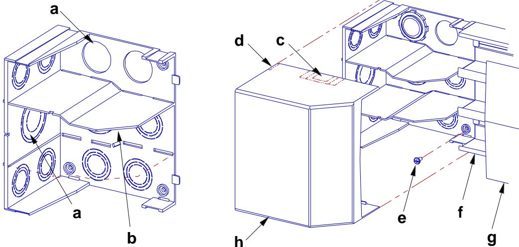
a. Remove knock-outs as required for end feed of back feed.
