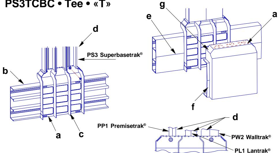
a. Remove knock-outs and appropriate openings for raceway as required. See General Information Note 4.
