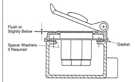
**Note:** Receptacle should be attached to box with spacers between the receptacle mounting strap and box flange (if required) so that the receptacle face is flush or slightly below the sealing surface of the wall plate (see Fig. 1).
