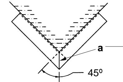
For lighting, power or Class 1 conductors: Miter cut required. For communications, Class 2, Class 3 or conductive Optical Fiber conductors: Square cut or miter is permissible.
