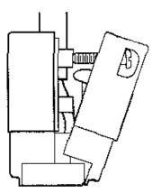
CLOSE OPEN SIDE. INSURE THAT CONDUCTORS REMAIN LOCATED IN PLACE BETWEEN SLOTS OF TERMINALS AND TIGHTEN SCREWS EVENLY UNTIL THE SIDE IS FULLY CLOSED.
