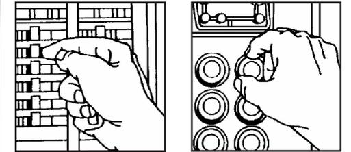
Next, plug in and turn ON the lamp or radio at the receptacle's other outlet to make sure the power is OFF at both outlets. If the power is not OFF, stop work and call an electrician to complete the installation.
