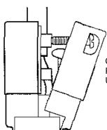
CLOSE OPEN SIDE. INSURE THAT CONDUCTORS REMAIN LOCATED IN PLACE BETWEEN SLOTS OF TERMINALS AND TIGHTEN SCREWS EVENLY UNTIL THE SIDE IS FULLY CLOSED.
