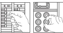
Next, plug in and turn ON the lamp or radio at the receptacle's other outlet to make sure the power is OFF at both outlets. If the power is not OFF, stop work and call an electrician to complete the installation
