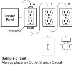
AFCI/GFCI in position A. All outlets of the protected branch, including lighting and receptacle outlets must be connected to the load side of the AFCI/GFCI
