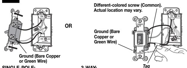
**SINGLE-POLE:** Insulated wires connected to two screws of the same color. Replace with a SINGLE-POLE dimmer. See Step 5a.
