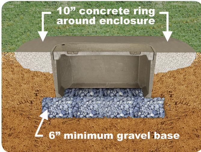
Concrete collars may be desired to give added protection to Hubbell enclosures installed by driveways, parking lots, and off-roadway areas that are subject to occasional non-deliberate traffic. Concrete collars are not necessary in grassy areas or areas subject solely to pedestrian traffic.
