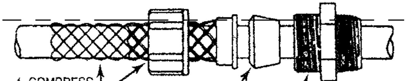
1. COMPRESS MESH END AND APPLY COMPRESSION NUT AND MESH ON CORD AS SHOWN.
