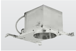
P821-AT Ceiling opening: 6-7/8" dia. Plaster frame: 8-3/8" x 13" Recessed depth: 7-5/8" Pryouts: 1/2" & 3/4"
