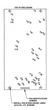
RESET PLATE HOLE KEY STARTER ONLY AND COMBINATION SIZE 0 AND 1 CATALOG NUMBERS B7011 & B7021
